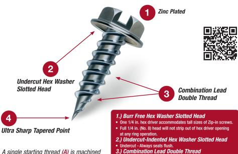
A single starting thread (A) is machined down to the very tip of the point and is the source of Zip-in's® penetrating power. The second thread (B) above the point engages after initial penetration and moves the screw through very fast.
