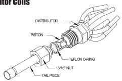
Fig 7A-1. Flowrator assembly components
