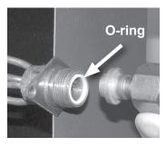
**I-5.** Taking care that the white Teflon seal is still in place inside the flowrater body, firmly seat the stub and screw the attachment nut to flowrater body.
