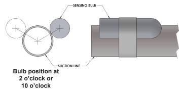
Fig 7B-2. Recommended location for horizontal TXV bulb mount
