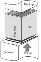
Air Flow Furnace Coil (both sides) Ductino
