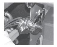
III-1. Disassemble the flowrator body using two wrenches. Unscrew the body with a counterclockwise motion.
