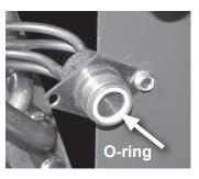
III-3. Replace the Teflon O-ring seal in place (located between the halves).
