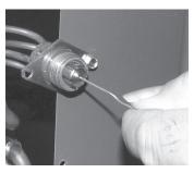
III-2. Remove the existing flowrator piston using a small wire or pick.
