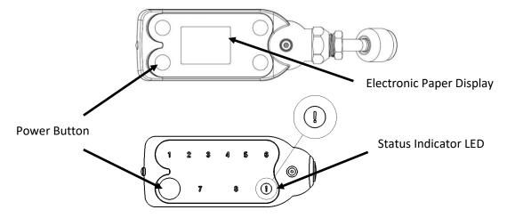
When using the YJACK PATH®, numeric LEDs 1-8 will illuminate to indicate the number of YJACK™, TITANMAX™ and P51-870 TITAN® devices within range.
