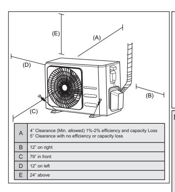
Refer to the following diagram to ensure proper distance from walls and ceiling:
