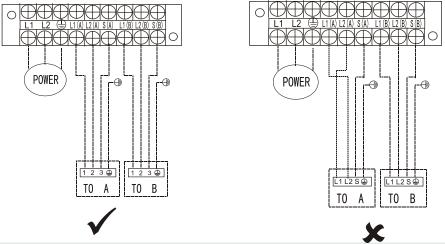
**NOTE**: Refer to the following figures if end-users wish to perform their own wiring. Run the main power cord through the lower line-outlet of the cord clamp.
