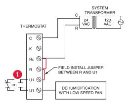
Fig. 226. Dehumidification with low speed fan using a variable speed blower.
