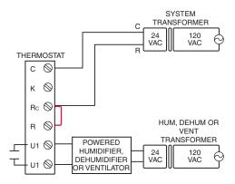
Fig. 225. Wiring a powered humidifier, dehumidifier, or ventilator.
