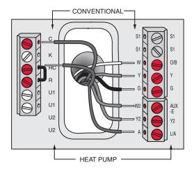
Fig. 13. Thermostat wired directly to equipment.
