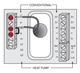
Fig. 14. Inserting wires in thermostat terminal block.
