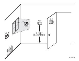
Fig. 9. Selecting thermostat location.
