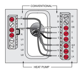
Fig. 222. Inserting wires in thermostat terminal block.
