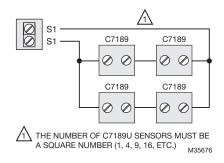
Fig. 231. Wiring 4 C7189U sensors.
