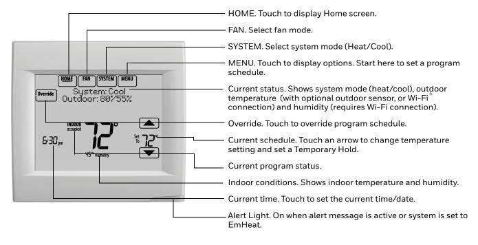
Fig. 29. Quick reference to commercial display.
