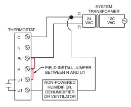
Fig. 227. Wiring a non-powered humidifier, dehumidifier, or ventilator.
