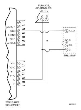
Fig. 230. Economizer control without economizer fault alert using TH8321WF.
