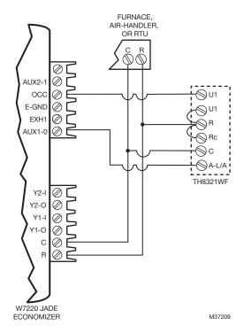
Fig. 229. Economizer control with economizer fault alert using TH8321WF.
