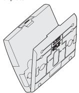
Fig. 10. Separate wallplate from thermostat.
