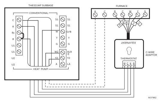
Fig. 223. Example C-wire adapter wiring diagram for a conventional application.
