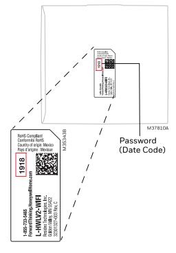
Fig. 2. Finding thermostat password.
