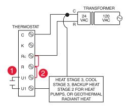
Fig. 228. Wiring a heat or cool stage to U1.
