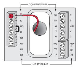
Fig. 12. Connecting C wire to terminal block.
