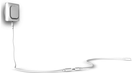
Fig. 1. Plugging in additional cable sensors.
